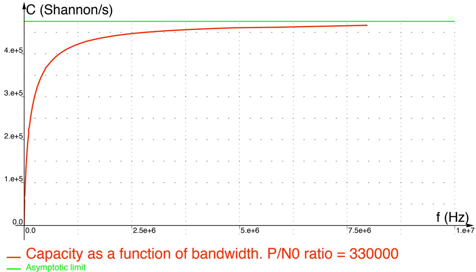
Capacity of band-limited channel with  $\frac{N_0}{2}$  noise power spectral density and signal power  $P$  :
