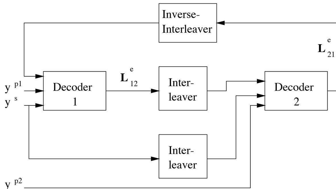
Decoders 1 and 2 use BCJR algorithm to compute the posterior probability of each source bit given the corresponding parity bits and prior probabilities of source bits.
