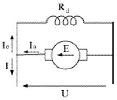
Self-starting is possible thanks to the remanent magnetization of the inductor
