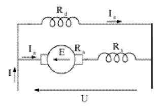
m.m.f. =  $n_d I_e \pm n_s I_a$ =  $n_d \left( I_e \pm \frac{n_s}{n_d} I_a \right)$ =  $n_d I_f$  Mixed excitation: shunt and series inductor wound on the same poles
