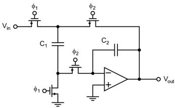
$<sup>^{3}</sup>H(z) = \frac{z^{-1}}{1 + c_2/c_1(1 - z^{-1})}, f_{-3dB} = \frac{1}{2\pi} \frac{C_1}{C_2} f_s$
