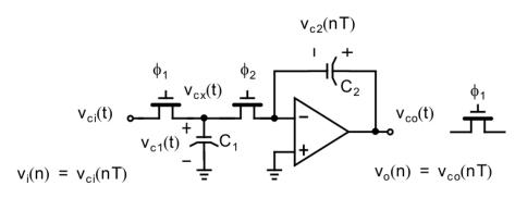
$$^{5}H(z) = -\left(^{C_{1}\!/C_{2}}\right)\left(^{A\!/A+1}\right)\frac{z^{-1}}{1-\left(1-^{C_{1}\!/C_{2}(A+1)}\right)z^{-1}},\ z_{p} = 1-\frac{C_{1}}{C_{2}}\frac{1}{A+1} \lesssim 1$$
