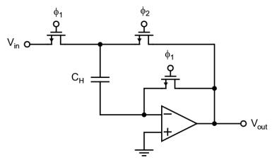
$$^{2}V_{out} = \frac{A}{A+1}V_{in} + \frac{A}{(A+1)^{2}}V_{offset}$$
