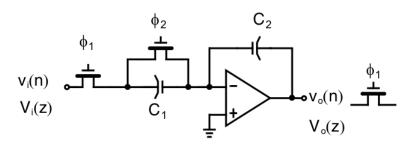
$<sup>^{4}</sup>H\left(z\right)=-\left(^{C_{1}}/c_{2}\right)\frac{1}{1-z^{-1}}$  (delay-free inverting integrator)
