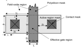
The n well surrounds the p-channel MOST, by at least  $3\lambda$ . The minimum spacing between the n well and the junctions of n-channel MOST is  $5\lambda$ . Therefore, the closest an n-channel MOST can be placed to a p-channel MOST is  $8\lambda$ . The minimum widths of poly, metal 1, and metal 2 are  $2\lambda$ ,  $2\lambda$ , and  $\lambda 3$ , respectively.
