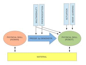
Fig. 1. In a PbD scenario, proprioception and multimodal sensing feed the adaptive mechanism, facilitating the transfer of skills for in-contact tasks from humans to robots. The material, rather than being an accessory entity, acts as the substrate that makes this transfer possible. Reinforcement learning, coupled to the capacity for action, completes the transfer by adapting the acquired skill to the robot's specific embodiment.
