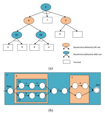
Fig. 2: An complex activity represented by (a) an AND-OR tree representation of a task and (b) the equivalent acyclic finite state machine
