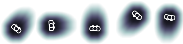
Fig. 4: Two-Gaussian mixture personal space model for individuals.
