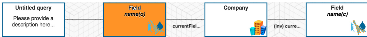
Fig. 18. A linear conjunctive query formulated by domain experts in the Statoil experiment.
