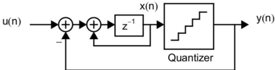
The state equations of the first-order  $\Sigma\Delta$  modulator are given by:
