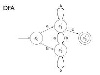
$\begin{array}{l} s_0' & \{1,2,5,6,7\} \\ s_1' & \{3,8,1,2,5,6,7\} \\ s_2' & \{8,1,2,5,6,7\} \\ s_3' & \{4\} \end{array}$
